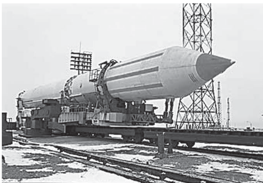
Fig. 24 Zenit-2 with Tselina-2 satellite (Kosmos-2369) on its way to the launch pad. (source: Federal Space Agency)
